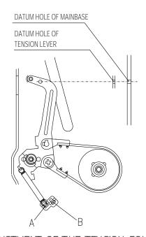
Fig.3-17 ADJUSTMENT OF THE TENSION POLE POSITION
